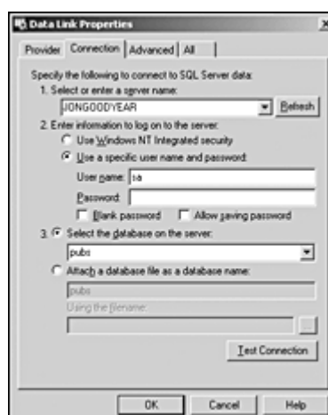
Figure 3.2. Dialog box used to set the properties of the data link file.
